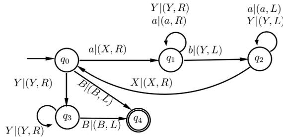
Figure 19.1: Transition diagram for TM accepting Language  $L = \{a^n b^n \mid n \geq 0\}$
