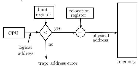
► When the CPU scheduler selects a process for execution, the dispatcher loads the relocation and limit registers
